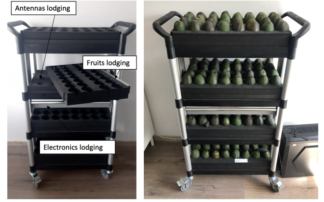
Fig. 6. Prototype of the smart trolley. Lodging for fruits, antennas and electronics are visible.
