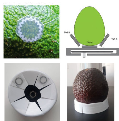
Fig. 5. Sensing tags for monitoring the ripening of the avocado . A tri-leaf shaped plastic support hosts the three tags and guarantees a firm position of the fruit all along the monitoring period. Tags are in contact with the fruit in three points.
